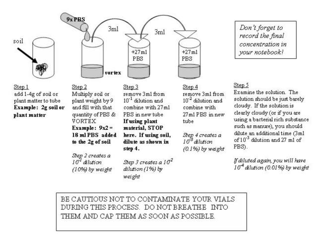
**Figure 2. Summary of steps to create the appropriate concentration.** The dilution series is created in order to achieve a final concentration of 1g of soil / 1000 g of final solution. The weight/weight dilution factors are commonly used in microbiology.
